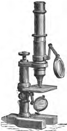
FIG. 16.—Stand III. of Hartnack, with joint and condenser.
